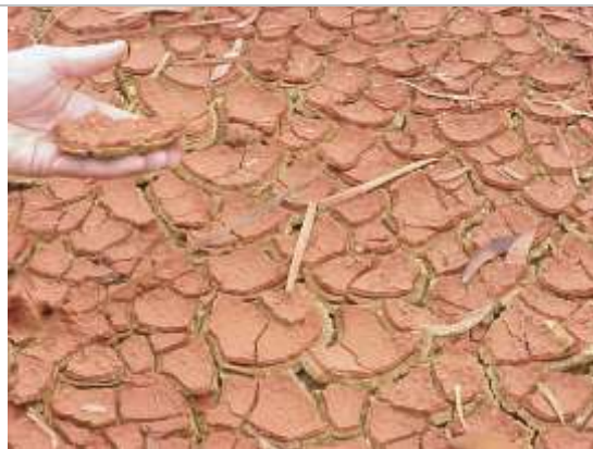
Figure: Sediment remaining after water treatment with red mud residue
