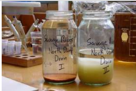
Figure: Similar contaminated mine waters after treatment with red mud residue and lime. Lime treatment (left) leaves behind large volumes of sludges which are difficult to deal with – red mud (right) residues leave behind sediments which can be used for farming.
