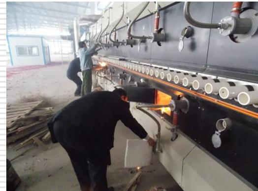
The glass ceramic sintering kiln
